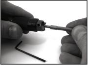
Step 2) For Hand Use: Insert the precision case length pilot fully into cutter head and tighten set screw with provided hex wrench.
