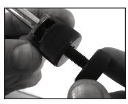
Step 1) Back-off lock screw on trimmer body and insert the shell holder for your caliber. Place a case in the shell holder and firmly tighten lock screw to securely hold the case.
