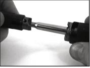
Step 3) Slide the pilot into the case and through the flash hole. (Note, cases should be sized and decapped before trimming.) Now simply turn the cutter until the pilot hits stop and no more brass is removed. Cases will be trimmed to exact length each time.
