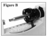
With the chuckhead lock still open, feed in the chuckhead shaft, with cartridge, so that the pilot enters the cartridge case neck and the cutter face is touching the case mouth. Tighten the chuckhead on the cartridge case by turning the knob handle clockwise.
