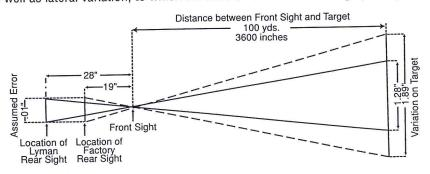
The diagram above shows how a longer "Sight Radius" affects the accuracy of your shooting. An average increase of 11" in "Sight Radius" translates into 32% greater inherent accuracy at 100 yards. This greater inherent accuracy is proportional to the target range, i.e., 32% at 100 yards, 64% at 200 yards, 128% at 300 yards etc. It is easy to understand why all match target rifles use a rear aperture sight mounted as far to the rear as possible.
