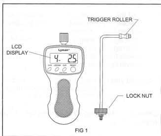
Using The Trigger Pull Gauge:
