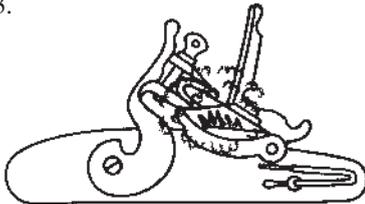
The hammer continues to fall and the direct blow of the flint against the frizzen changes to a heavy scraping of the frizzen by the flint. This produces a shower of sparks which start the ignition of the priming powder.
