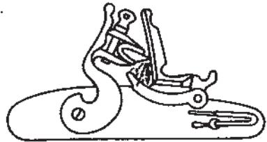
As the hammer falls, the leading edge of the flint makes initial contact with the face of the frizzen. The continuing force of the hammer starts to rock the springloaded frizzen back and up on its pivot. Sparks generated here are minor and probably offer very little to the ignition process.
