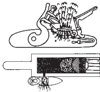
The priming is fully ignited and the main charge has just begun to burn. Typically, there will be a certain amount of the main charge pushed up the barrel a ways behind the ball before the powder is consumed.
