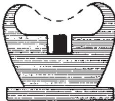
**Primitive Rear Sight**—This is a traditional one piece, fixed sight which allows final shape and elevation adjustments to be filed into it by the shooter.
