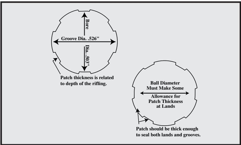
We know the ball must be smaller than the bore diameter so let's select a .498" diameter ball as the best choice for this bore.
