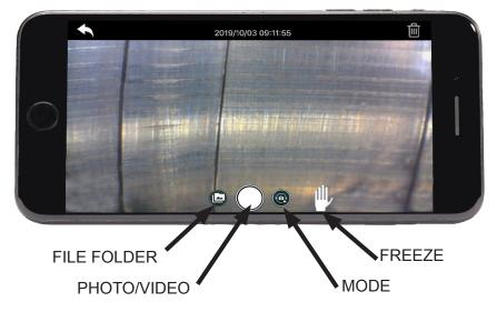
Taking a photo: simply press the Photo/Video button at the bottom of the APP, or quickly press the button on the handle of the Borecam. You can also "freeze" an image for review by pressing the Hand button on the APP. The APP will then allow you select Save or Cancel. Save will storage the image in your File Folder, Cancel will return you to the live image.
