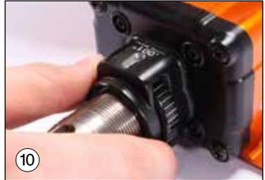
6. To remove the cutter head, first turn the Adjustment Wheel clockwise until the Adjuster Barrel is free of the main body. (pic 10)
