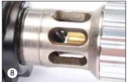
TRIMMING TIP: when setting the initial cutting depth make sure you have fully compressed the spring; repeat this step a few times, to ensure the proper initial setting.
