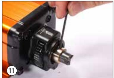
7. Locate the set screw on the brass cutter housing. (pic 11) Loosen set screw, and remove cutter. Use caution when working in the cutter head area, the carbide cutter is very sharp and can cause injury.
