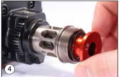
2. Place the bushing into the adjuster barrel as shown (pic 4) with the bushing number facing you. Reinstall the bushing cap and tighten.
