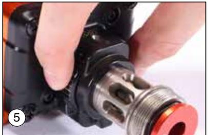
A viewing window is located at the top of the adjustment wheel housing, this window will allow the user to view the graduation marks to ensure a proper setting.
