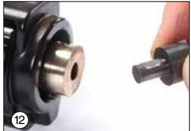
8. To install a new cutter head, first locate the "flat" on shank of the cutter head. (pic 12) The "flat" should be inserted so that the set screw will contact it when tightened. Tighten set screw firmly.
