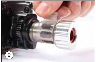
4. Turn your trimmer on to the highest RPM setting. Insert a sized case into the Bushing. Using light, even pressure move the case forward towards the cutter. When the case makes contact with the cutter, use firm pressure but do not “JAM” the case into the cutter. This will cause rough, inconsistent cuts, which could damage the case or cutter head.
