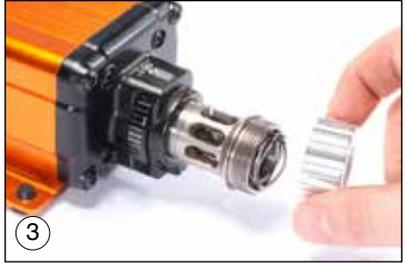
1. Select the proper bushing for the caliber you are trimming. Unthread the bushing cap (pic 3). Under the bushing cap you will find a compression spring, this spring must be installed in order for the trimmer to function correctly.
