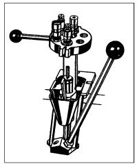
and position it against the edge of your bench top in the most convenient location, usually near the center of the bench, leaving a work area on each side of the press. Mark the position of the mounting holes and drill them; then, using %" bolts and suitable washers and nuts, securely anchor the press.
