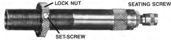
Select the Bullet Seating Die which is pictured as number four in illustration A. Back off the bullet seating screw and screw the die body into the threaded portion of the tool handles.
